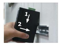
Step 2: Place the bottom of DIN rail lightly into the track.
