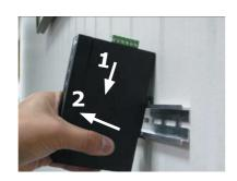
Step 5: Lightly pull out the bottom of DIN rail to remove it from the track.
